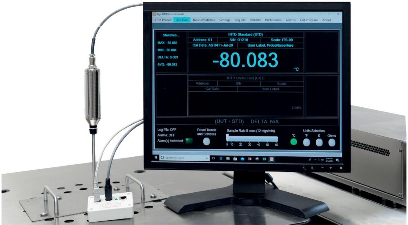
The Kaye IRTD is a high accuracy traceable temperature reference standard used with Kaye Validation systems while calibrating sensors. The broad temperature range from  $-196^{\circ}\text{C}$  to  $420^{\circ}\text{C}$ , with an accuracy of  $\pm 0.025^{\circ}\text{C}$ , enables it to be used in virtually all temperature validation applications and high-end calibration labs.
