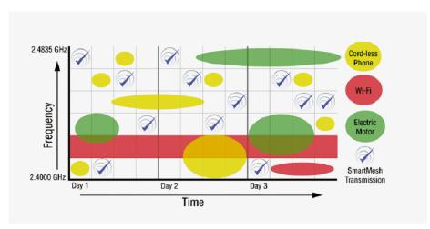
Frequency hopping ensures reliable transmission
