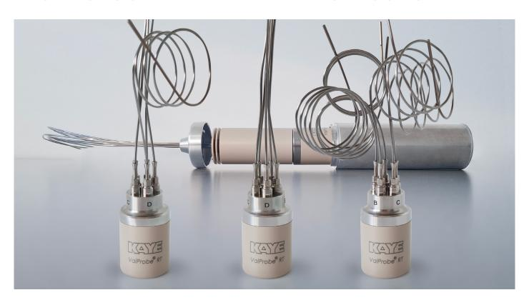
The real-time Kaye ValProbe RT data loggers, obtainable in one and two sensor versions, are now also available with five sensors in conjunction with bendable probes.
