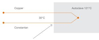
Temperature gradient of 91°C between the inside wall and the outside.
