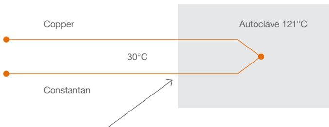
Temperature gradient of 91°C between the inside wall and the outside.
