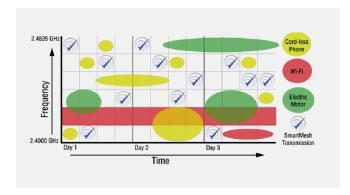
In addition the mesh protocol permits the system to learn about the RF environment and dynamically adjust the network parameters to best fit the current situation. The network provides an accurate time reference for the whole network, ensuring all loggers and the base station are time synchronized correctly. Each data sample is timestamped with this network time.
