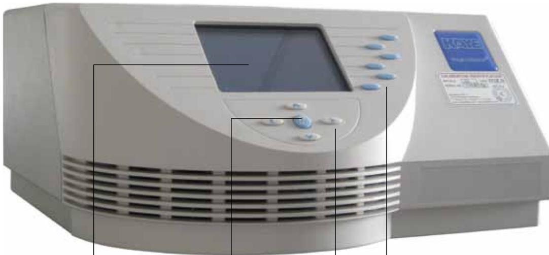
Displays online data and calculations, set-up parameters and sensor offsets.
