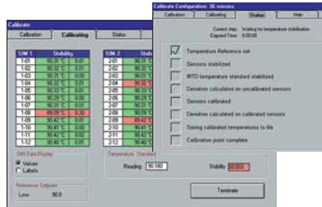
The PC shows the entire calibration process on one screen. Data fields change color to show the progress of stability and deviation for each sensor. A status screen (above, right) lists each step and indicates where the system is in the process.
