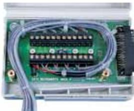
A secure path for wiring sensors is provided for strain relief and organization of your probes. The wired SIM shows 10 thermocouples and one pressure sensor (a shunt resistor is used by the Kaye Validator for converting current to voltage). You can order SIMs pre-wired with thermocouple probes, labeled numerically.
