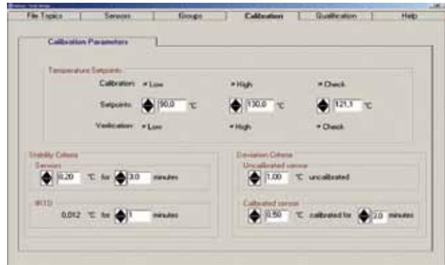
Set the criteria for a sensor calibration—low, high and check point for the actual calibration and the points to verify calibration after a study.
