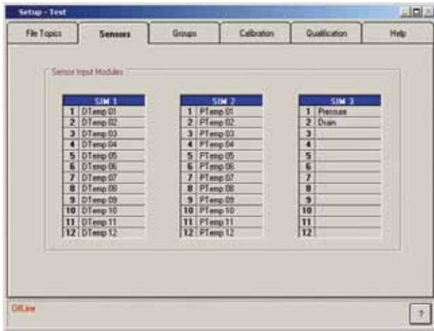
The set-up screen shows all defined sensors in the set-up. Clicking the Groups tab lets you select the sensors you want to include in a particular group.
