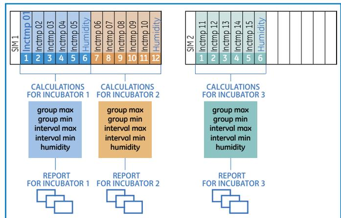
Users can add unlimited cycles, separating qualification data into separate process phases, and up to 25 groups, with their own calculations and graphs during reporting, often eliminating the need for post-processing in Excel®.
